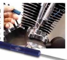
No. 746 - Use on most hydraulic tappets, OEM and aftermarket, for Twin Cam or Evo. (Does not work on Solids, JIMS Hydrosolids or other limited travel tappets)
