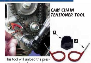
sure on the primary and secondary chain tensioners to assemble and disassemble cams. This tool also checks spring loads on chain ten-
