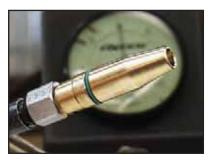
cially designed super grip finish that will keep teflon or k-line style seals in place. We have also shortened the top of the guides for high lift cams to clear all valve spring collars. With Manganese Bronze Alloy, intake guides can be fit to .0008" and exhaust guides can be fit to .0012" or more depending on application - when used with JIMS® valves only.
