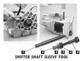
Use to remove and install the shifter shaft sleeve in all 5 & 6 aftermarket speeds. This tool may be used to remove, install replacements, or upgrade shifter shaft sleeve, assembly, and drum. For more details see No.1664-IS instructions.
