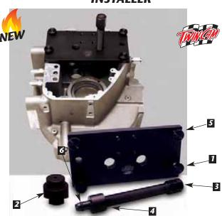
Use this tool to press in, and install, the two inner cam bearings JIMS® No.8991K. This tool has been designed to press from the letter side of the inner cam bearings, by putting all the pushing pressure to the very outer wall of bearing shell. Eliminats any damage to the bearings, cam and cases. This tool will stop at the case and set the bearing depth to .023" to .028" below the case surface. Use with JIMS® Tool No.1279 to remove bearings. For more details see No.787-IS instructions.
