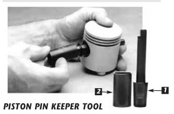
For installing and removing split "L" ring keepers. For more details see No.2368-IS instructions.
