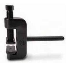
this special tool. The chain manufacturers have determined a press fit adds strength to the connecting link and should always be used.
