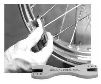
This tool fits 6 nipple sizes. From 1 to 6. Made by Rowe®.
