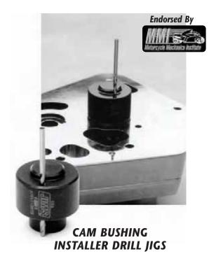
Just press in new JIMS® cam bushing with jig and drill through guide hole in jig, through both bushing and cam cover. Press in new staking pin No.2201, and bushing is locked in place. Jig comes complete with instructions. Use to install and drill dowel pin hole in cam bushing to the factory specification. Supplied with drill.
