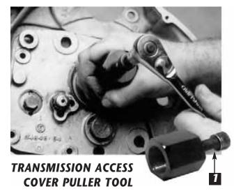
Use to remove transmission access cover which is press fit on two dowel pins. For more details see No.95560-IS instructions.
