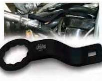
Hiro came to us with a great flat rate time saver stem nut tool for use on Touring Model Harleys. Normally to get access to the top stem nut you would need to remove the radio package. With this tool you are able to loosen, tighten and torque to spec. the 1-1/2" stem nut without radio removal and ultimately saving you 45 minutes for an experienced mechanic! For more details see No.977-IS instructions.
