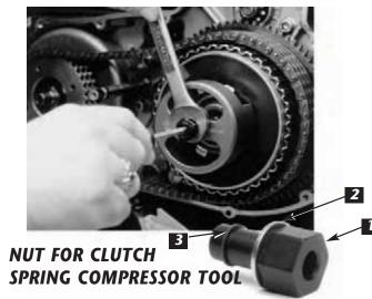
Use to release clutch spring for ease of retainer ring removal and installation (Must be used with No.38515-90 Main Body). Available Separately. For more details see No.2285-IS instructions.
