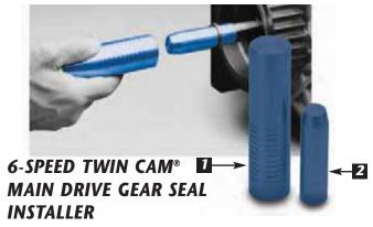
This tool is designed to properly align and install to the right depth, the main drive gear seal, H-D® No.12077 into the end of the gear. This can be performed while the assembled transmission is either on a bench or in the motorcycle chassis. For more details see No.972-IS instructions.
