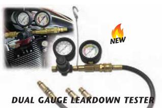
Includes a 12mm and a 10mm adapter. Cages comes with protective rubber cover. The hose assembly has both 14mm and 18mm spark plug threads. The tool is easy to use and will troubleshoot cylinder leakdown issues such as valve seat issues, bad rings, bad head gasket, etc. For more details see No.782-IS instructions.
