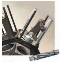
JIMS® wrist pin bushings. Reams are easy to use with their designed lead in taper at the start of each ream. Use JIMS® No.1284 Rod Clamp tool. For more details see No.1726-IS instructions.
