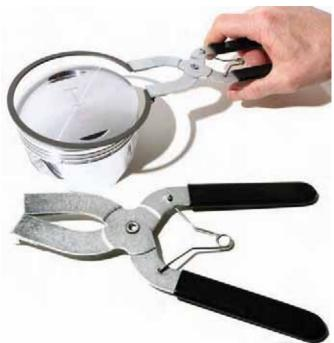
Use to remove and install piston rings. Reduces the risk of ring breakage. This tool has tappered jaws to hold all normal size rings from 3/64" to 1/4" (1.2 -6.3mm) thickness.
