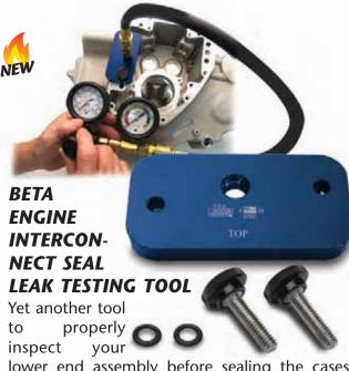
lower end assembly before sealing the cases. This new tool will check the sealing of the interconnect seal H-D No.45359-00. Use the tool along with a JIMS No.782 Leakdown Tester. This test assures you there is no leakage in the seal that can cause over oiling of the lower end. For more details see No.780-IS instructions.
