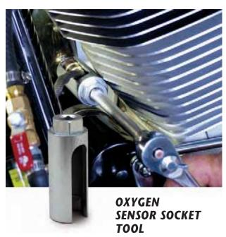
This tool is used to remove or install the oxygen sensor on all closed loop fuel injected H-D® models. Socket has a 3/8" drive receiver or can be used with a 7/8" wrench. Socket will withstand up to 125 ft/lbs of torque.
