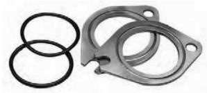
(Head to Manifold Spacer) Use with Stroker Kits when fitting standard width manifolds and using taller cylinders. Also use with IIMS® 113" or 116" Stroker's using +0.100" taller cylinders. Spacers kits will increase the distance (wider) between the heads by 0.080", allows the use of standard width manifolds such as the standard Harley® EFI, Screamin' Eagle®, S&S® or other stock width manifolds having standard size intake ports. For more details see No.721-IS instructions.
