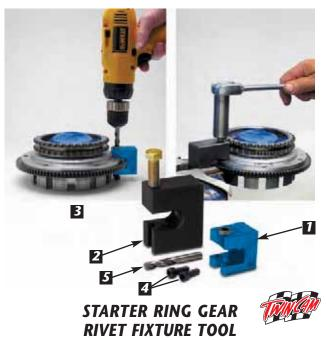
This tool is designed to remove the starter ring gear rivets from Big Twin clutch shells to install JIMS® No. 639 and 640 or equivalent performance starter ring gears. For more details see No.965-IS instructions.
