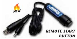
This simple remote switch makes it easy to activate the starter & rotate the engine without starting. Comes in handy for tappet adjustments, servicing and diagnosing starting & electrical issues. Tool provided with four foot lengths well insulated lead cables with an alligator clips for positive and one for negative post hookups. For more details see No.752-IS instructions.
