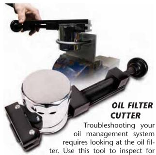
any damaging particles that may be trapped in the filter. This tool locks down the filter for a clean cut around the filter base by rotating the filter. Use this tool with JIMS® No. 934 oil filter cutting stand along with a common vise. See left side. Will fit filters up to 5-1/2" diameter.
