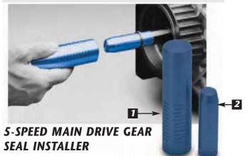
Use to install the main drive gear oil seal to the proper depth with transmission assembled. Comes with a protective sleeve for seal. We recommend using IIMS® seal No's.12013A & 12035A. The sleeve can also be used when installing transmission assembly to protect main drive gear inner bearings. For more details see No.2256-IS instructions.
